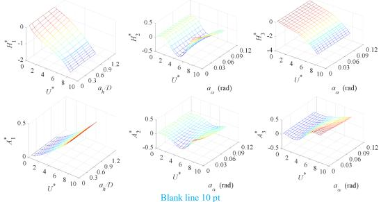
**Figure 2.** Identified results of the major flutter derivatives ( $\alpha_e = -5^\circ$ )
